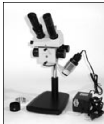
Figure 4—The microscope can also be mounted on the base that comes with it to be used as a standard inspection scope. The 1.5x Barlow lens and adapter ring (lower left) are not installed in this case. (The production adapter ring has a black anodized finish.)
