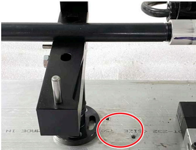
FIGURE 18—The red oval shows the mounting holes.
