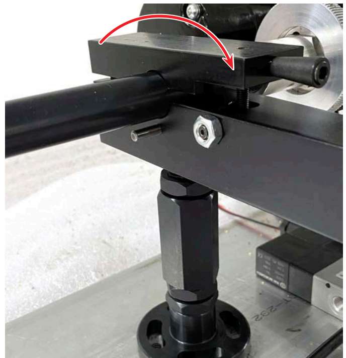
FIGURE 21—The red arrow shows the direction to close the top clamp of the front-mount assembly.
