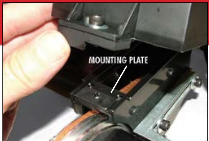
FIGURE 17—Insert the mounting plate between the belt guard halves and secure the speed control housing to the nut in plate.
