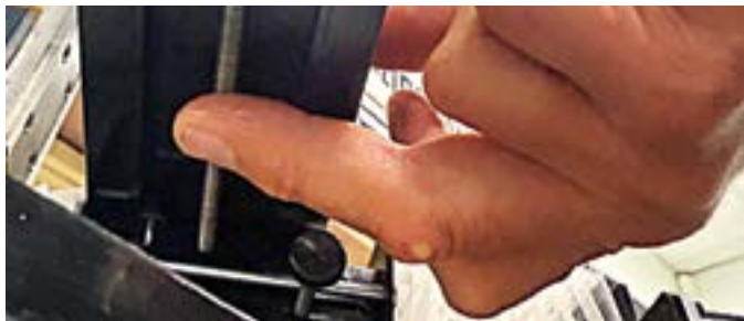
FIGURE 4—Use a light oil and spread it regularly across all screw threads. Shown on the underside of the mill table.
