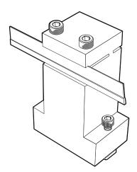
NOTE: Always use plenty of cutting fluid when using the Cutoff Tool.
