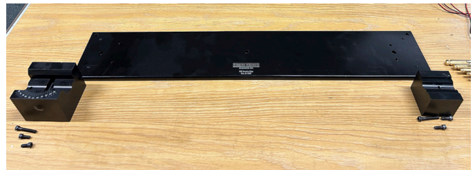
FIGURE 4—The assembly parts for the new lathe base (44050).
