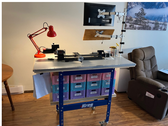
FIGURE 1 —The touchscreen monitor and keyboard for CNC control are seen in stowed position. In use, they are swung to the right and assume the normal right-hand position for CNC work. The lower shelf holds plastic storage crates for all the accessories.
