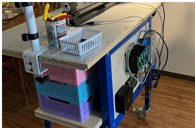
FIGURE 2 —The CNC motion controls, mounted on the back of the workstation includes a mini PC, HiCon Integra 4-motor controller with motor drivers. The control software will be Mach4, which integrates perfectly with the Integra motion controller hardware.
