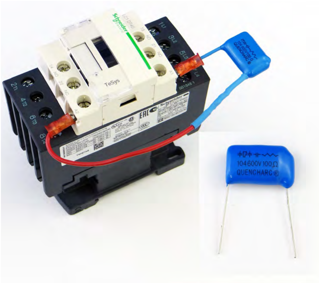
Contactors with snubber installed across the coil
