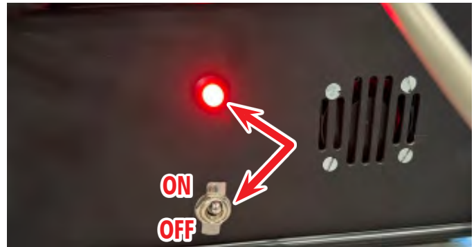
FIGURE 35—When the Sherline/Acorn CNC Controller power is on, the red LED light will illuminate.
