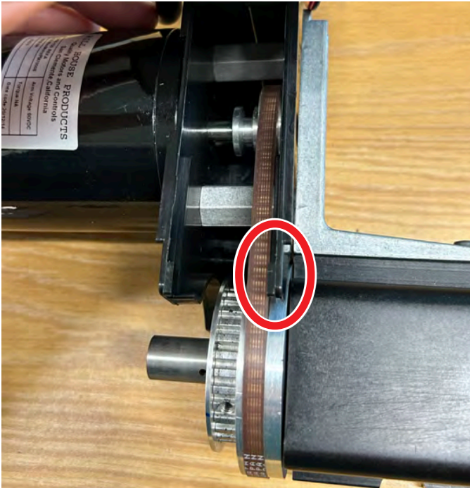
FIGURE 13—The red oval indicates the front ear of the plastic belt guard.
