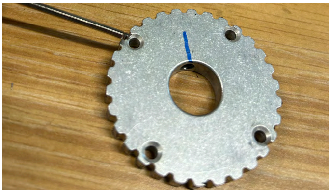
FIGURE 5—P/N 43220E is the 30T cog pulley for the #1 Morse headstock. P/N 43223E is the 30T cog pulley for the 3C headstock.
