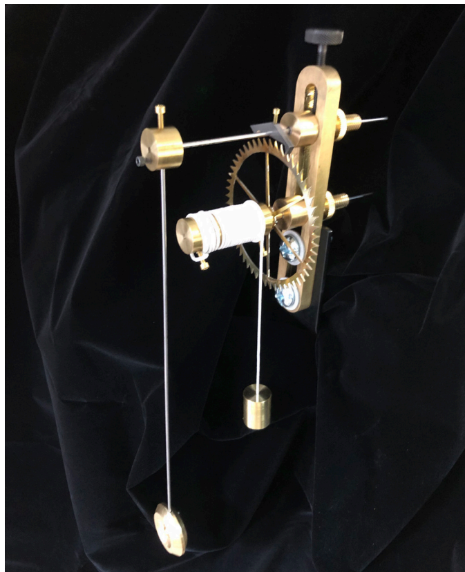
FIGURE 5—This is David’s escapement test setup. Both the pallets and escape wheel were cut on his Sherline Accu-Pro mill.
