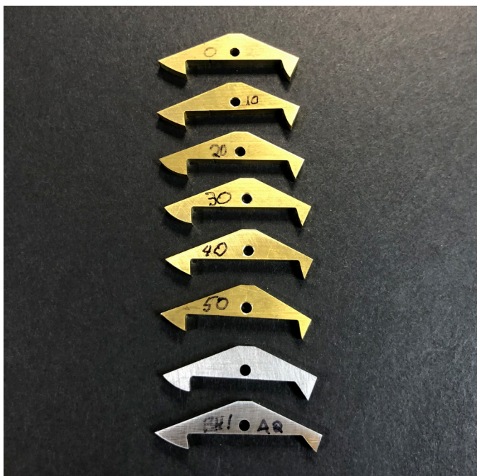
FIGURE 4—These are a set of test pallets made for the large clock. David machines them first in brass, which cuts quickly. He then finds the best one, and can make an identical copy using the CNC program in A2 steel. Cutting it in steel takes a day or so. The brass ones can be cut in a few hours.
