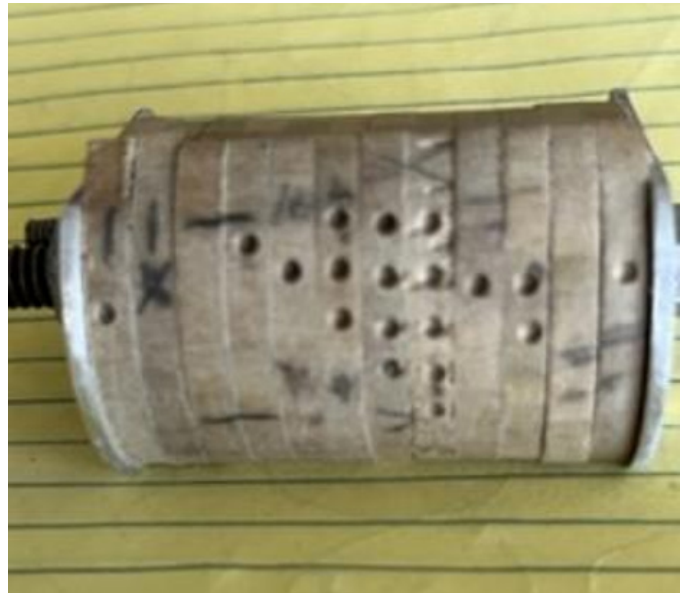
FIGURE 6—Balance hole in webs.
