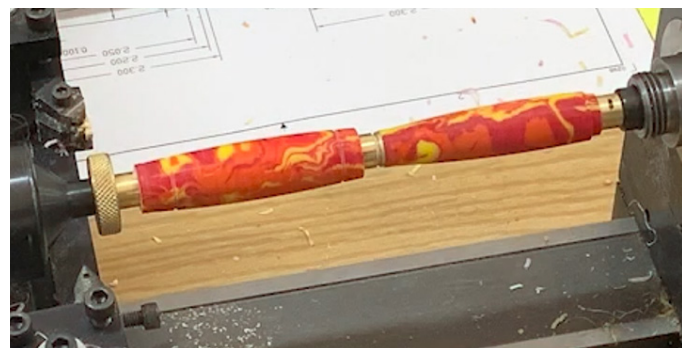
FIGURE 13—Turning pen parts on a Sherline CNC lathe.
