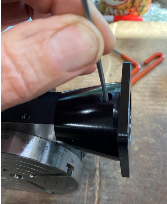
FIGURE 2—The 3/32" Allen wrench inserted through the access hole is used as a brake to keep the coupling from moving while you are tightening the button head screw (P/N 37200).
