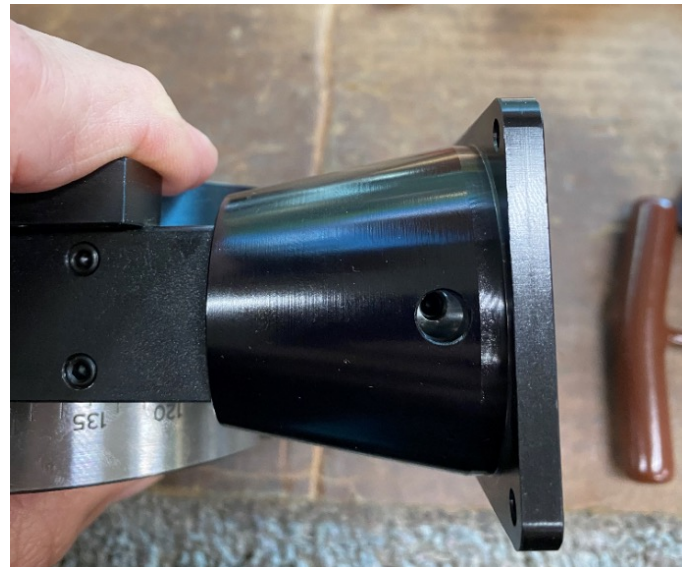
FIGURE 1—Shows the set screw aligned with the motor mount access hole.
