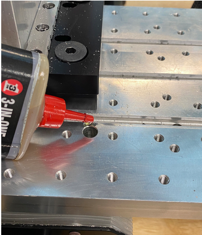
FIGURE 3—The saddle oiler access hole on the tooling plate.
