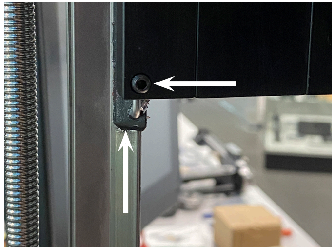
FIGURE 11—The arrows are pointing to the Z-axis mill set screw and gib.
