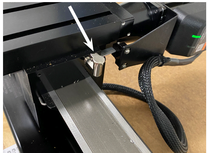
FIGURE 2— The arrow is pointing to the oiler reservoir on the lathe saddle. The reservoir cover on the ball screw lathe is a spring-loaded, hinged cap.
