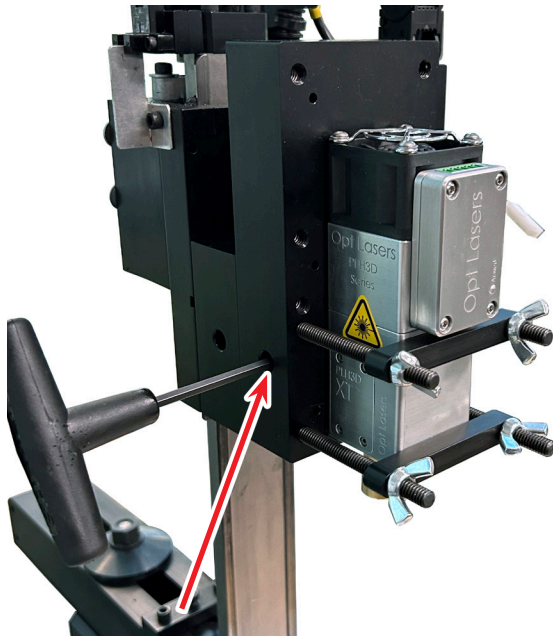
FIGURE 7—The red arrow points to the access hole for the laser mount set screw.
