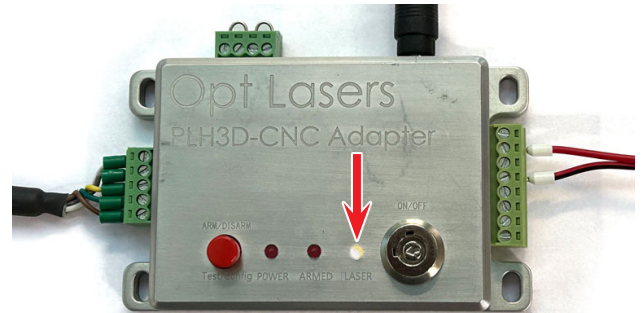
FIGURE 13—This is what you see when you turn the Laser on. Note that the Laser LED is lit before the Power LED.
