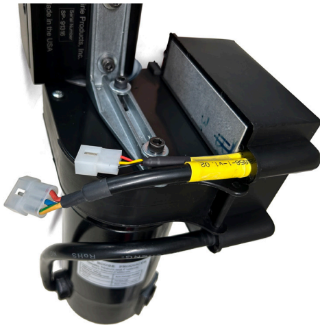
FIGURE 3—Wires with connectors leading out of the motor and speed-control unit.
