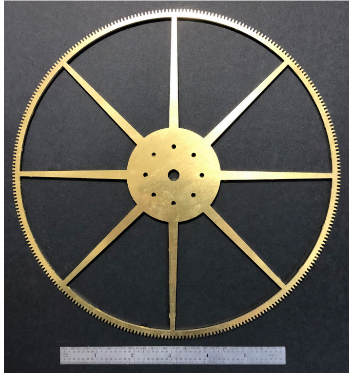
FIGURE 1—The wheel is 8.6" in diameter and the machinist's rule is 6" long. Photo credit: Dave Bishop.
