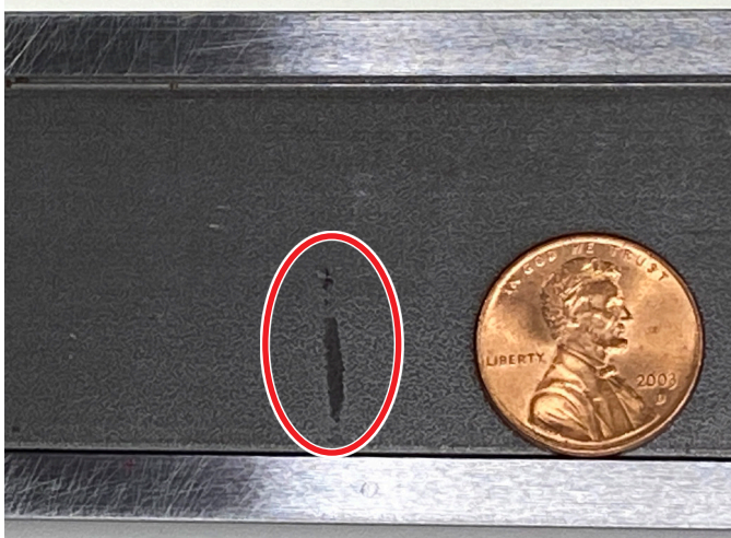
FIGURE 1—Example of an extrusion dent.
