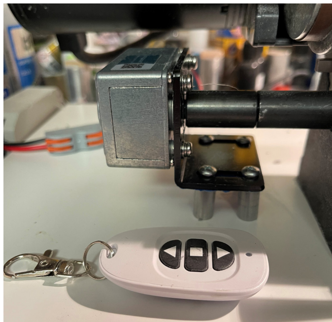
FIGURE 3— The power-feed motor is on the backside of the controller, and it fits nicely beneath the headstock DC motor.
