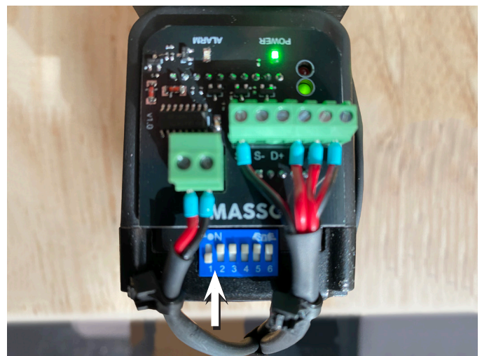
FIGURE 3—The arrow shows the location of the dip switches inside the stepper motor power supply.
