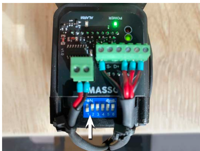
FIGURE 74—The arrow shows the location of the dip switches inside the stepper motor power supply.
