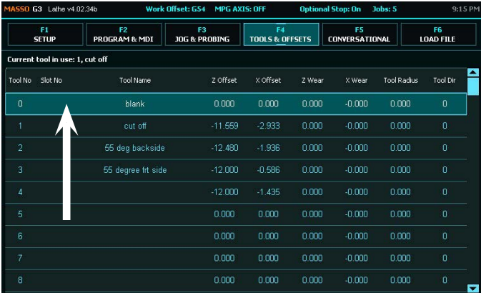
FIGURE 49—Always leave Tool #0 X and Z Offset values as Zero. Name it “blank.”
