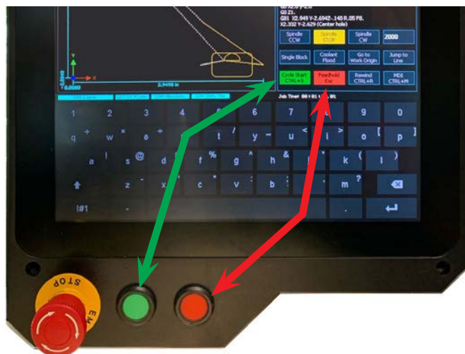
FIGURE 75—The green arrow points to the Cycle Start buttons and the red arrow points to the Feedhold buttons.
