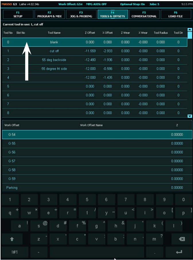
FIGURE 40—Always leave Tool #0 X and Z Offset values as Zero. Name it “blank.”
