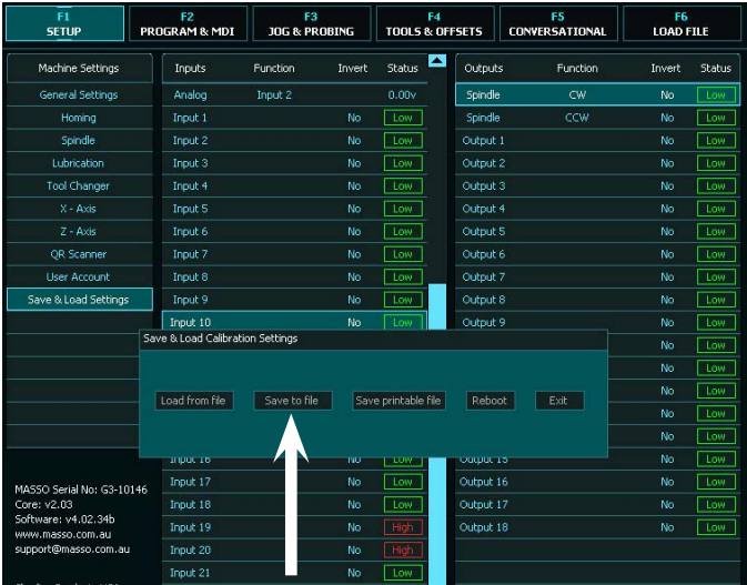
FIGURE 48—Touch “Save to File” and all of your settings and tool files will be saved to the USB drive.
