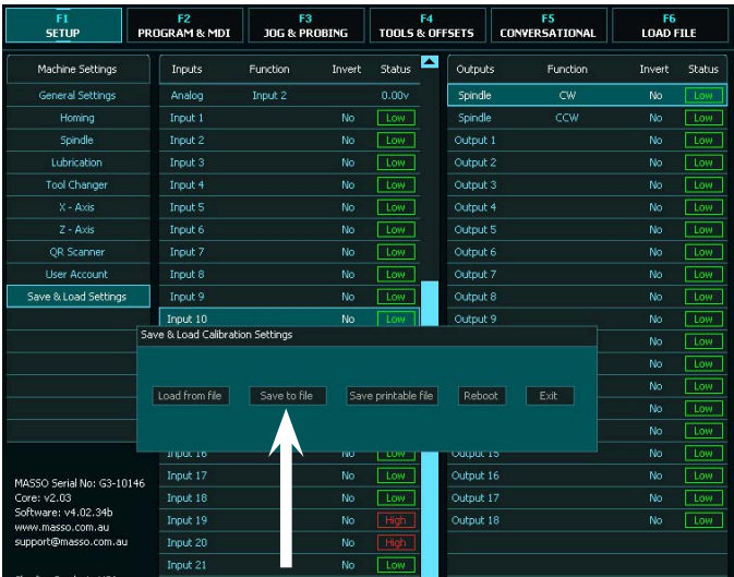
FIGURE 39—Touch “Save to File” and all of your settings and tool files will be saved to the USB drive.
