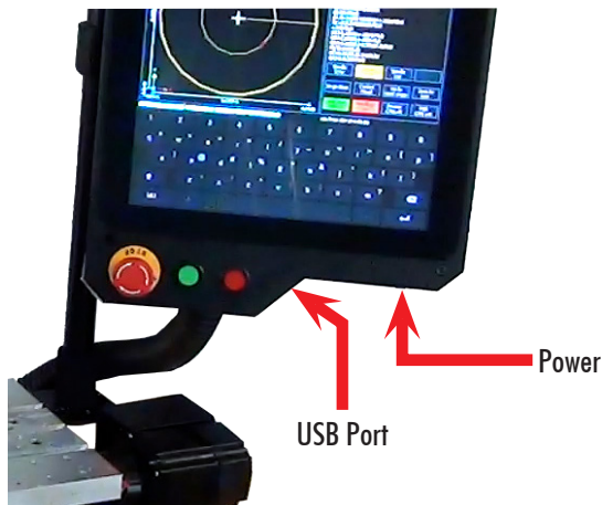
FIGURE 1—The red arrows show the locations of the Power and the USB port at the base of the monitor. See Figure 75 on page 19 for the functions of the buttons on the bottom of the monitor.
