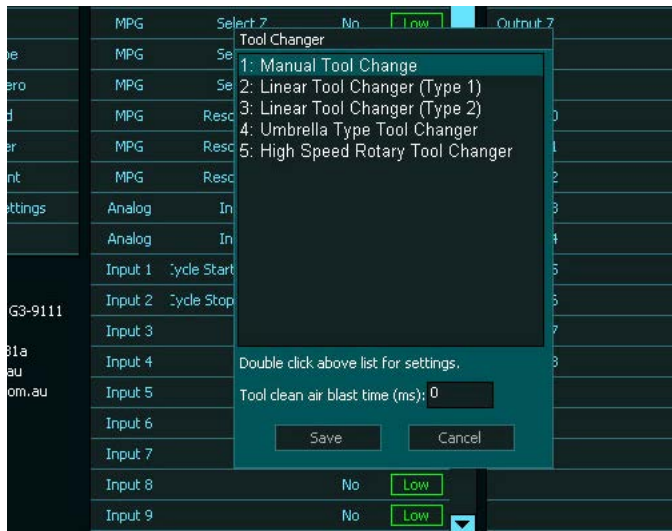
FIGURE 53—Tool Changer mill dialog box. Make sure you select the Manual Tool Change function.
