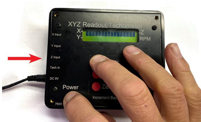
FIGURE 5—Plug the power cord back into the DRO display in the direction of the red arrow while holding down the buttons.
