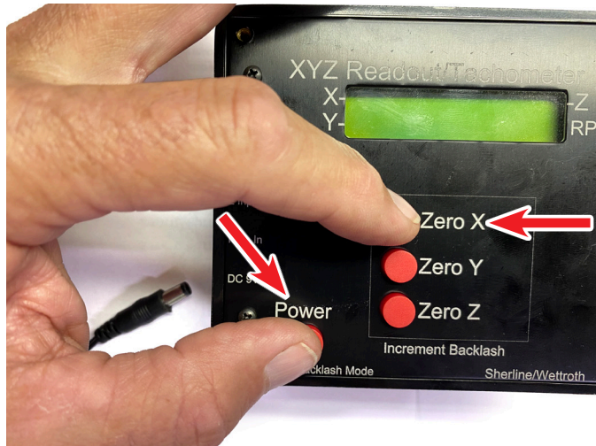
FIGURE 4—The red arrows indicate that the X button and the Power button are pushed simultaneously.
