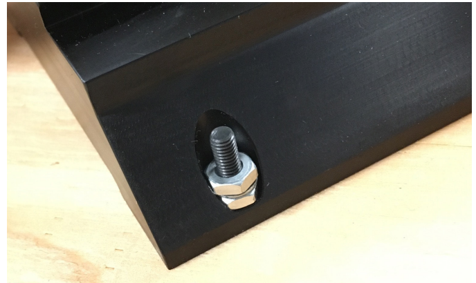
FIGURE 2—Shows the second locking nut and washer.
