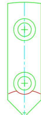
**SMALLER DIAMETER PIN INTERRUPTED-RADIUS CUT**
