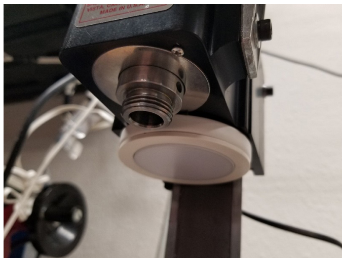
FIGURE 1—This photo shows the light installed under the headstock and spacer block.
