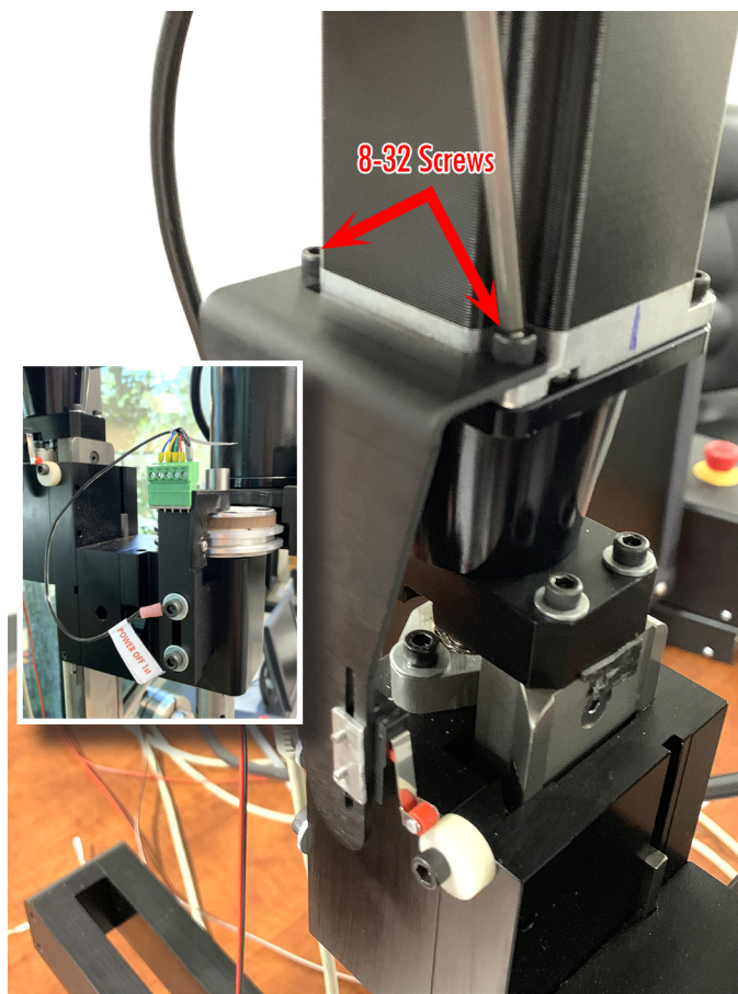
FIGURE 19—Install the Z-axis limit switch mounting bracket using the two 8-32 screws from the stepper motor.
