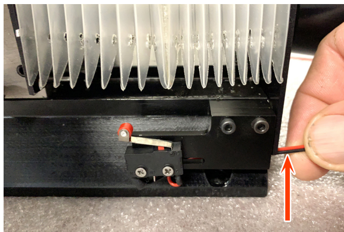
FIGURE 7—The limit switch mounted the with wires going between the mounting bracket and the mill base.
