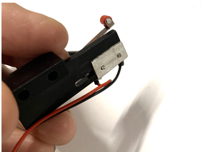
FIGURE 4—Y-axis limit switch assembly with the backing plate P/N 68046 attached.
