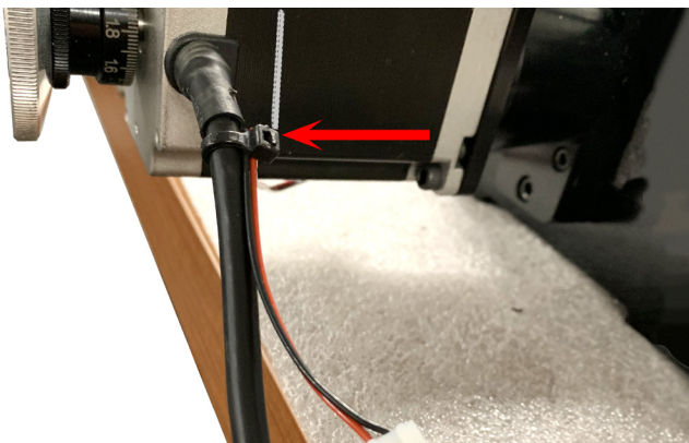
FIGURE 27 —Use wire cutters to trim off the excess zip tie flush at the knuckle. Exposed zip tie ends will cut you, so trim them flush.
