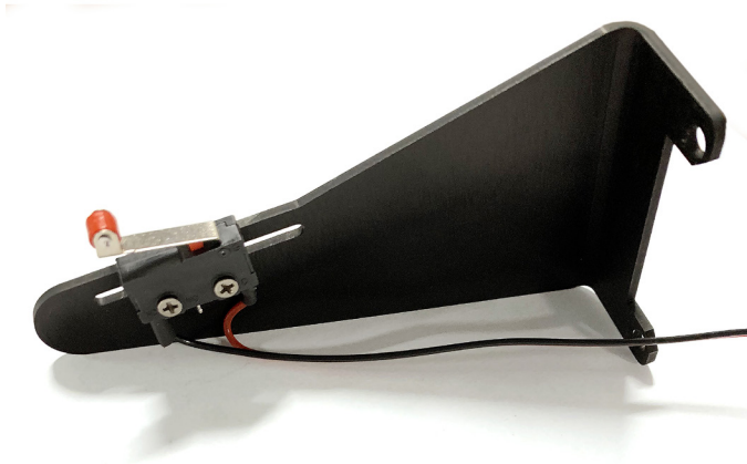
FIGURE 16—Limit switch mounted to the Z-axis limit switch mount.
