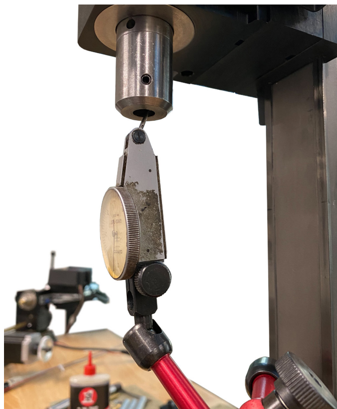
FIGURE 6—The indicator tip located inside the end mill holder from another angle.
