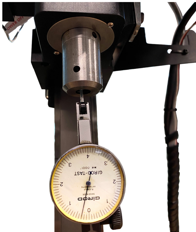
FIGURE 5—The indicator tip is located inside the 3/8" bore of the end mill holder.
