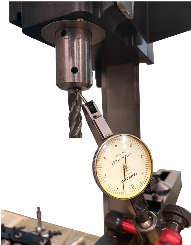
FIGURE 8—The indicator tip is located on the end mill shank.
