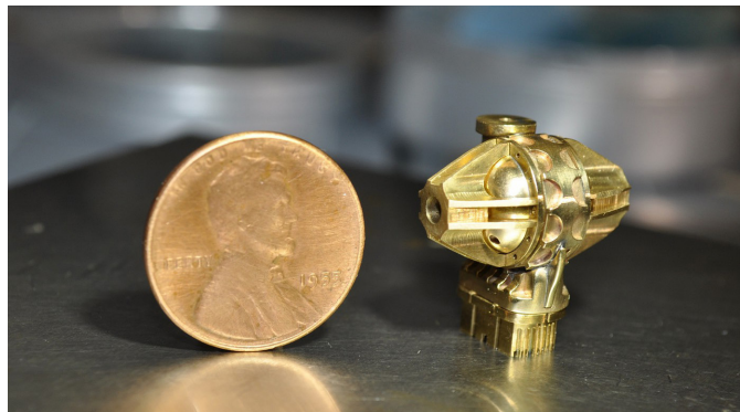
FIGURE 9—Close-up of the brass, quick-change rear end.
