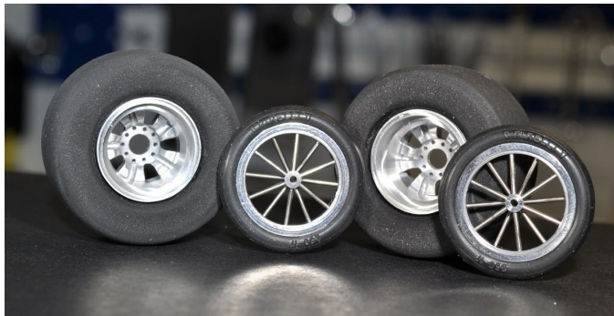
FIGURE 8—Machined wheel examples.
