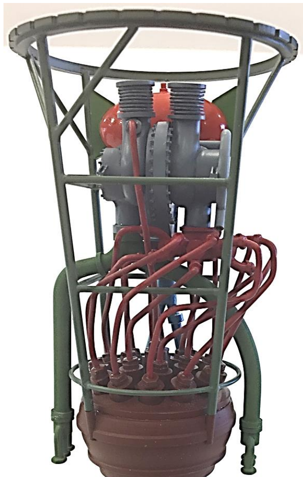
Figure 10 – Thrust Cage Assembly
