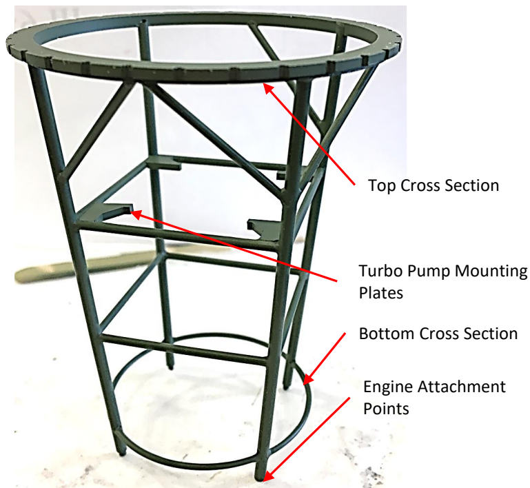
Figure 8 – Thrust Cage
