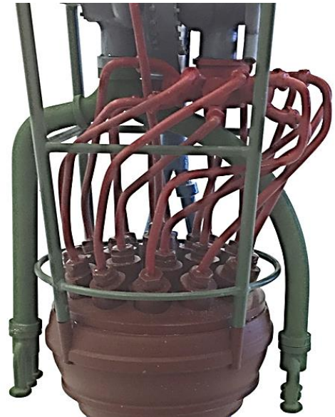
Figure 20 – Actual Alcohol Distribution Assembly Upper View
