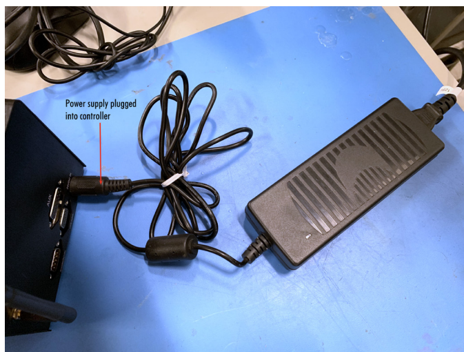
FIGURE 3—Connect the power supply to the controller.
