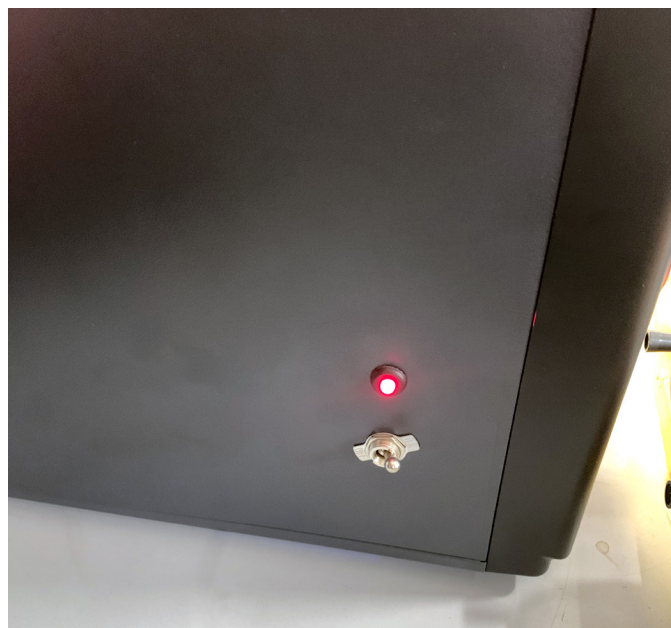
FIGURE 5—The red light indicates that the power is on to the driver box.
