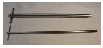
Two different size tap handles are shown. The top one is 13/32" in diameter and fits inside the Sherline spindle itself, while the smaller one at 1/4" diameter is for use with a WW collet holder. Fitted into the end of each shaft is a cut-off clock key providing the square hole for the end of the tap. (The apparent curve in the shaft is caused by the wide angle lens.)
