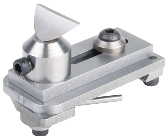
FIGURE 1—Sherline's W. R. Smith T-rest. A T-rest is used by watchmakers to support a hand-held cutting tool called a "graver." World-renowned watch- and clockmaker, William R. Smith designed a T-rest especially for the Sherline lathe that clamps to the lathe's bed in seconds.
