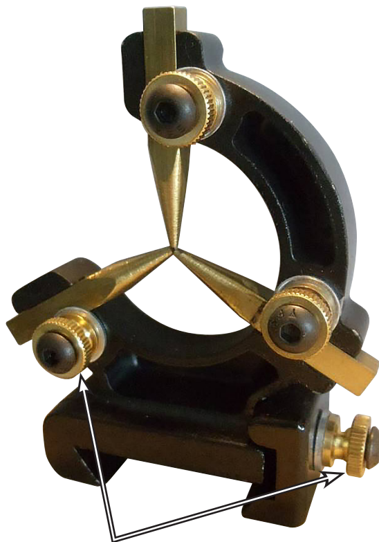
FIGURE 2—Knurl nuts were added to enable removal and adjustments by hand versus using an Allen wrench.
