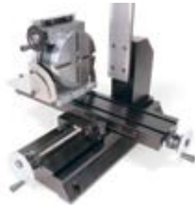
3700-OP Rotary Table set up on a 3750 Tilting Angle Table.
